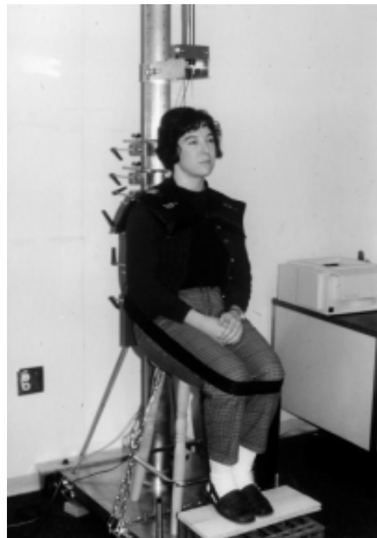
Fig 4. Stadiometer with subject in place and weights on shoulders.
